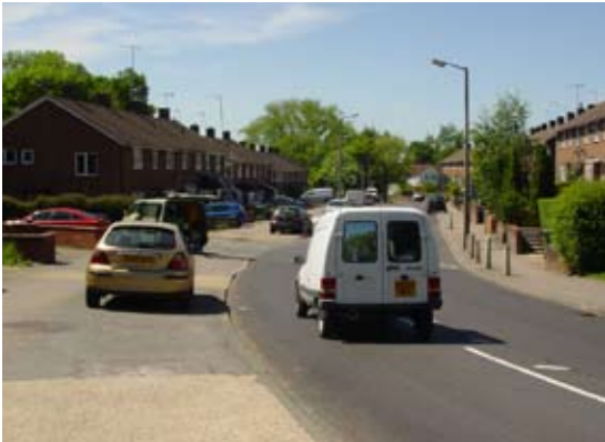
Bennetts End in Hemel Hempstead has some design flaws, such as poorly planned car parking that can block pavements and footways. These issues need to be designed out in the new neighbourhood.
